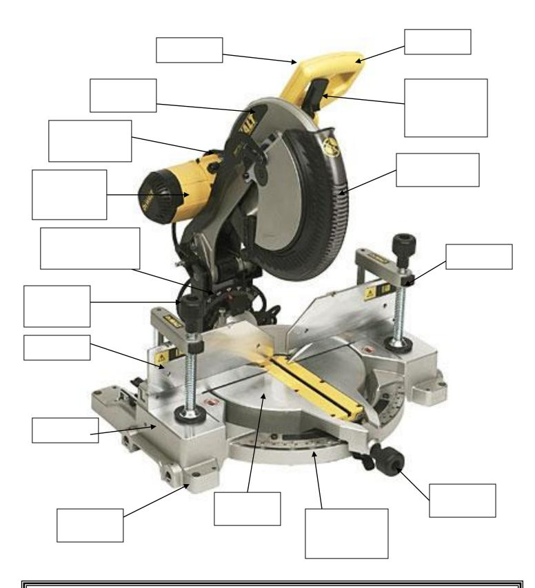
Base, Base footpads, Bottom saw guard, Bottom saw guard release lever, clamps, Dust extraction point, Fence, Handle, Locking handle, Motor housing & ventilation, Pillar locking lever, Scale of degrees for bevelling, Scale of degrees for mitring, Swivel base, Top saw guard, Trigger.
